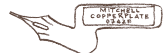
An elbow nib (here by Mitchell) can be inserted into a straight holder.
